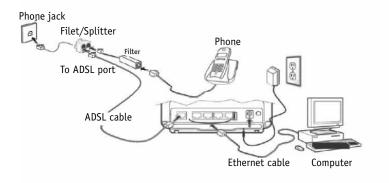
**Important note:** If you are plugging in or adding phones, it is very important to have a filter in place with ADSL technology.
