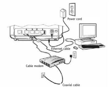
**Important note:** The Cable modem must be connected in the #4 port of your wireless modem router.
